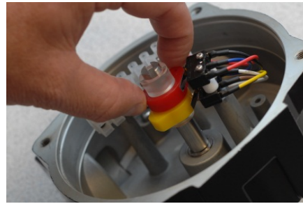
Red Cam Adjustment – Fully Closed
