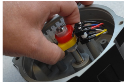
Yellow Cam Adjustment – Fully Open
